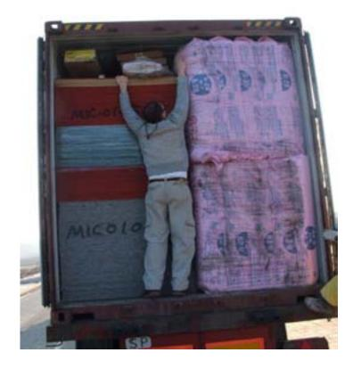
Note the eye hooks on the end of each panel above. Used to remove panels from the container.
